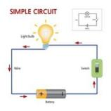
The current flows from negative to positive. There are no gaps so it is a complete circuit and the bulb lights up.
