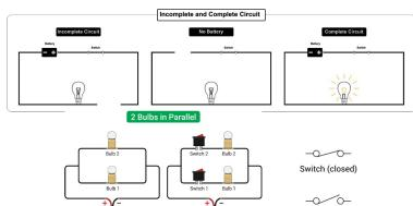
Switches can be placed in a parallel circuit, so that 1 light can be turned on while another is off (just like in a house).
